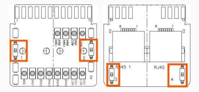
If more than 1 Slave inverter is connected there are no DIP Switches that need to be set,
