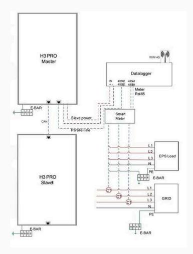
When doing parallel installations, only the Smartlogger/EMS has a CT/Meter connected, as it will control the power output of the Master and Slave inverters accordingly.
