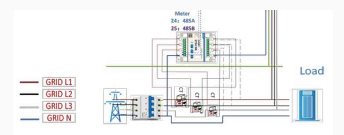
Insert L1/L2/L3/N wires ,CT and RS485A/B cable into the meter.Please refer to the meter wiring diagram on side of meter itself.
