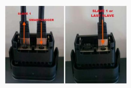
If more than two inverters are being installed then from the Master Inverter's CAN RJ45-2 to Slave 1 RJ45-1 then RJ45-2 to Slave 2 RJ45-1 and so forth
