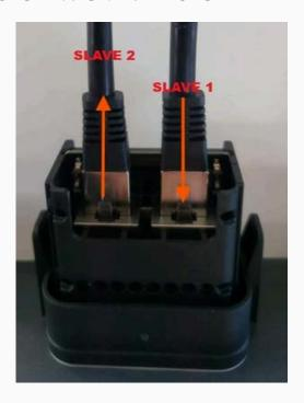
As pictured, the communication cable should go from the 'Parallel 2' port on the Master Inverter to the 'Parallel 1' on the 1st Slave Inverter, and so on for each Slave Inverter.
