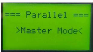
This will need to be changed to **Master Mode**Once this has been changed the Master Inverter will display Master and the Slave Inverter/Inverters will display **Slave 1, 2 ......**
