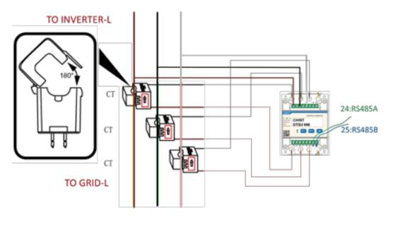
Notes: The 2,5,8 of the CT meter are connected to the three live wires L1, L2, and L3 respectively.
