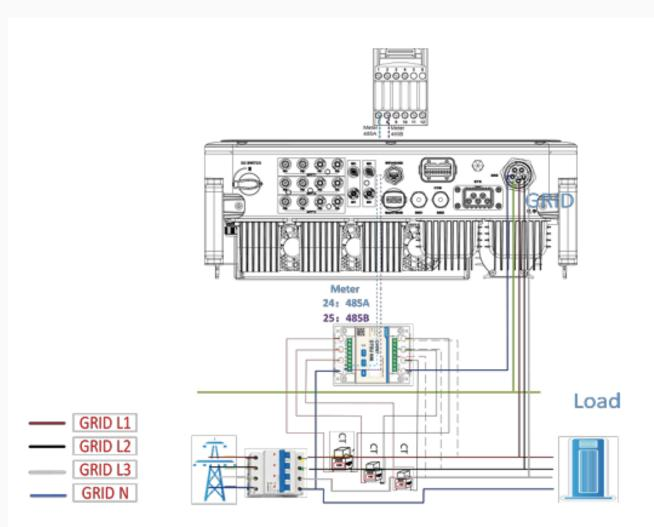
Insert L1/L2/L3/N wires ,CT and RS485A/B cable into the meter.Please refer to the meter wiring diagram on side of meter itself.
