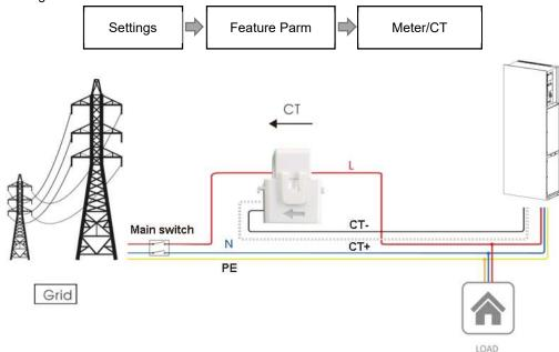
If there is another generator in the home, CT2 can be used to record the power generated by the generator and transmit the data to the website for monitoring.
