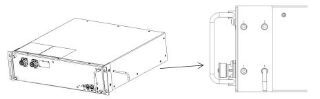
Push the battery into the All-In-One as shown in the figure below.
