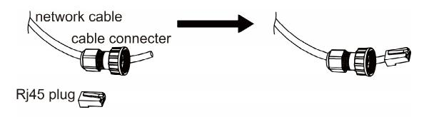
Step 4: Insert the cable connector into COM port at the bottom of energy station and screw it tightly. Then insert other side of the network cable into PC or another device.
