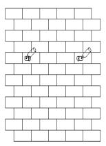
Drill holes on the marks with a diameter of 6mm drill. Insert the expansion screws into the hole.
